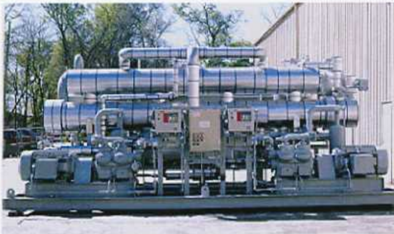
R22, 248 Ton Dual Process Refrigeration Unit controlled by two FES MicroMaster panels and insulated with polyurethane with stainless steel jacketing.
